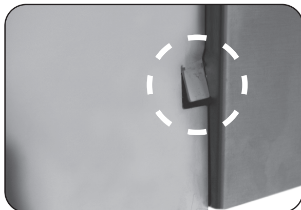
Fig. 25-3 Tab slightly bent in for clearance
